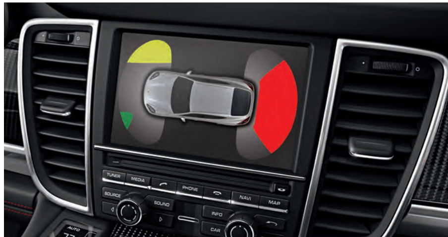
Graphical display of ParkAssist (front and rear)
