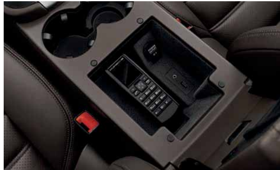
Telephone module with Bluetooth® handset
